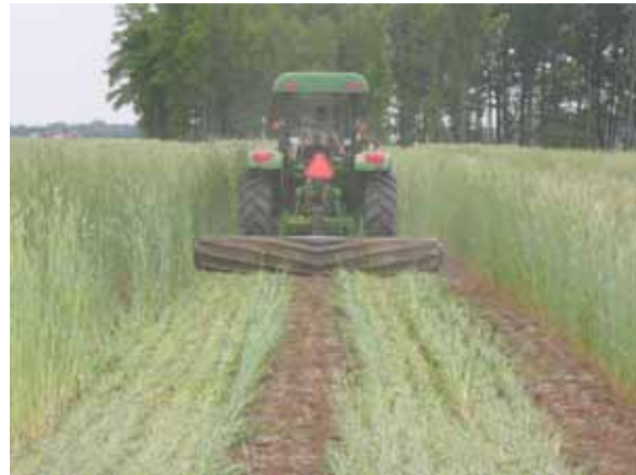
Picture 1. The roller/crimper knocks down cereal rye zone where burned down earlier to plant pumpkins.
